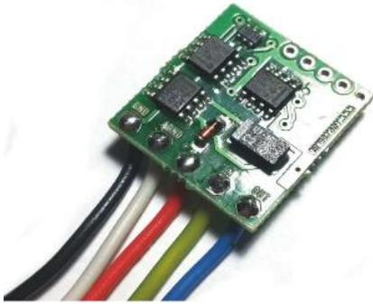
The electronic emulator of the catalyst could be used in case of removing vehicles' catalyst with two lambda probes/sensors (before the catalyst and after it). This module is installed in the open circuit of the second lambda probe. This does not require any reprogramming of the engine control units (ECU/ ECM), the entire system is operating in normal mode, and diagnostic is fully preserved. Microprocessor is the main part of the emulator.
