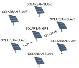
Use the learning button to scan drives and save coordinates. The button is available only when the GPS has determined the coordinates and there is no movement of the drives. When you press the knob, a short confirmation tone will sound.
